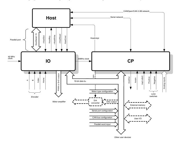
The IO chip contains the parallel host interface, the incremental encoder input along with motor output signals that are configured as PWM or step and direction signals according to the motor type selected for each axis.
