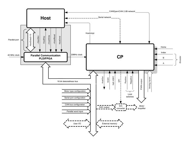
The shaded area shows the CPLD/FPGA that must be provided by the designer if parallel communication is required. A description and the necessary logic (in the form of schematics) of this device are detailed in the section Parallel FPGA section of this manual.
